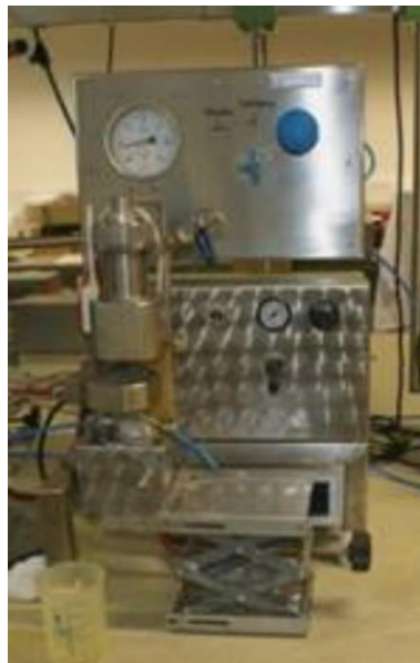
Figure 6. Laboratory equipment used to make the first filtration tests.
